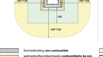
wall/ceiling/floor/attachments combustible/to be protected substitute insulation material calcium silicate (Promasil 950-KS) heat protection panel (accessories)
