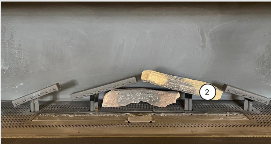
4. Position log no. 1 (with the recess) on the middle left burner as shown in the picture.
