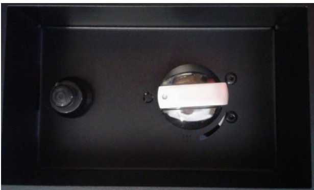
Photo 10 – Unscrewing the battery slot
