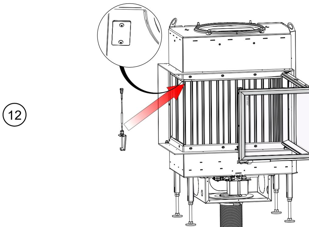
Variants cable routing - Thermocouple: right side or left side
