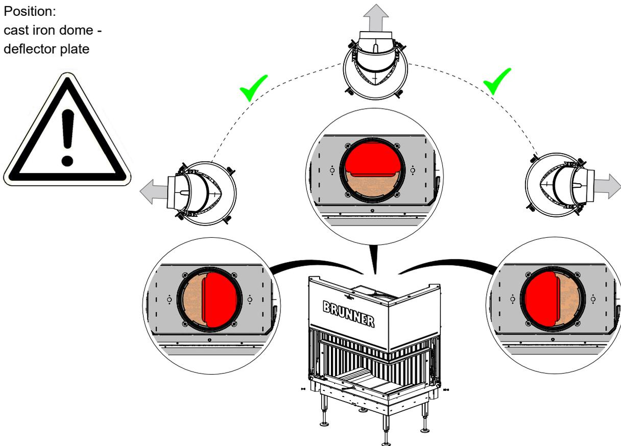
Examples for the position of the deflector plate : Connection variant for exhaust gases:
