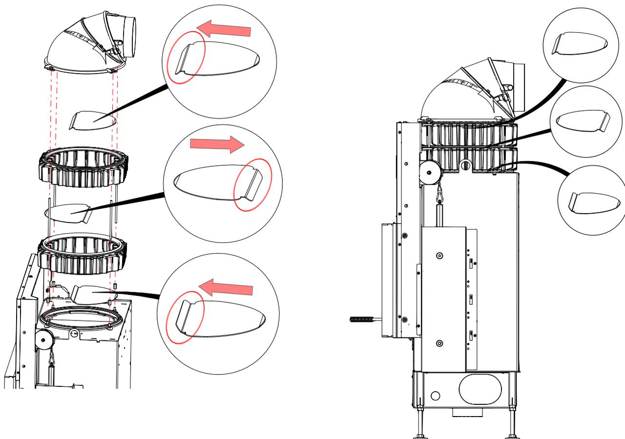
**Principle of flue gas routing with heat exchanger rings**
