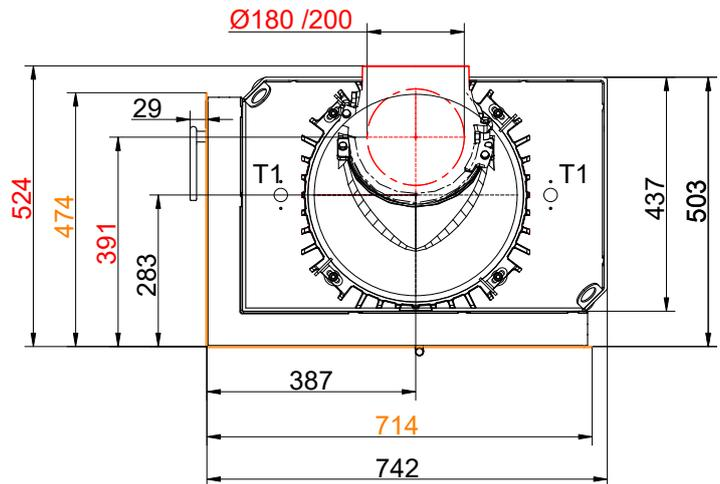
... left with door frame and cast iron heat exchanger rings + dome (side-opening door, DT)
